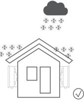
If conditions permit, we suggest to install snow retaining equipment for the inverter or installing the inverter in sheltered places or indoors.
